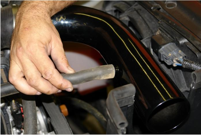
Step 10. Re-install the crankcase vent tube, and re-connect the electronic air sensor plug.
