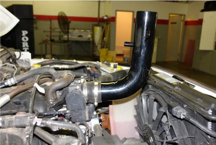
Step 7. Install electronic air sensor into grommet in new intake tube.
