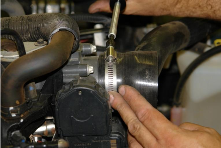
Step 5. Install new rubber reducer adapter
