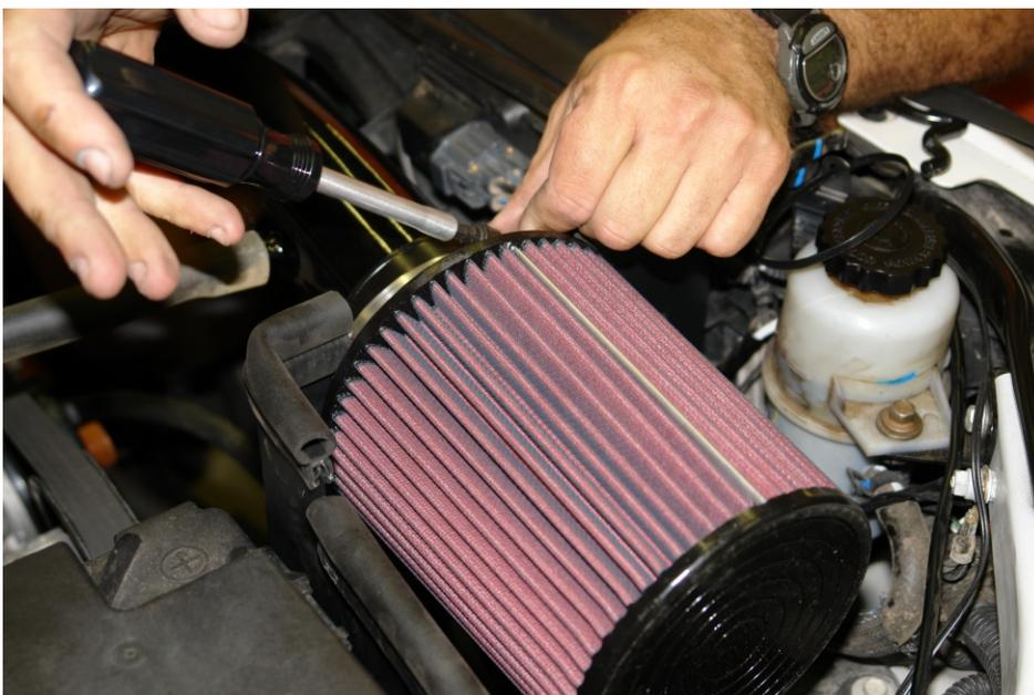
Step 11. Slide the air filter element into place and tighten clamp.
