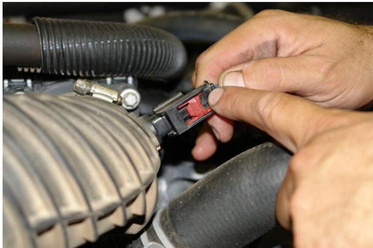
Step 3. Remove complete airbox assembly, including air intake tube,
