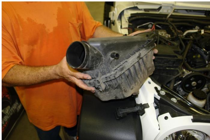
Step 4. Airbox completely removed, ready for re-installation
