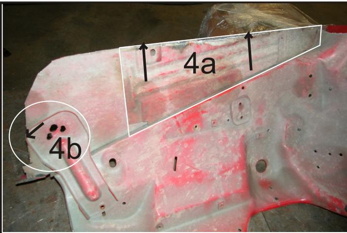
4. On the underside of the fender, you will see that a portion of the fender is double layered.
