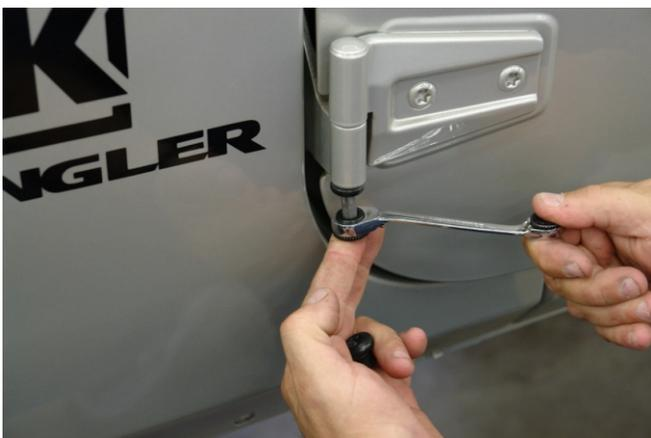
Step 4. Begin to remove the doors from vehicle, one side at a time. Unplug wire loom and remove door straps from retainer hooks.
