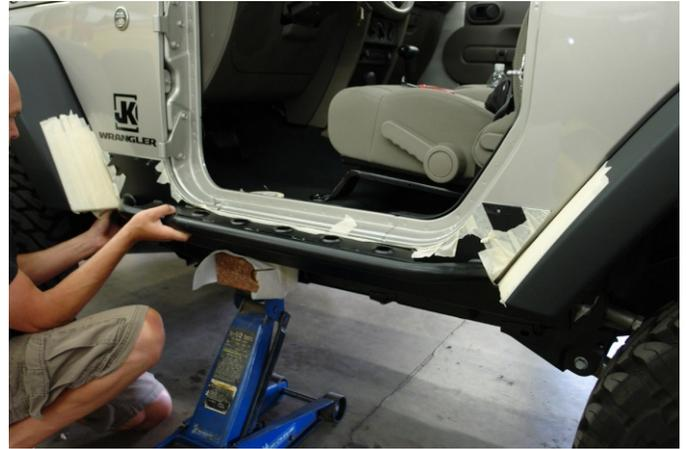
Step 11. Use a scratch awl to scribe a mark through the mounting holes at all points along the side rail.
