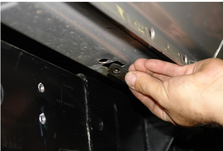
Step 6. Install nut clips into pockets on floor area. Shown below are the 8mm x 1.25" bolts supplied in the hardware kit.
