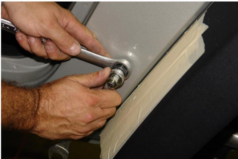
Step 25. Use the supplied tool to install the 1/4 -20 nut-sert at the rear upper edge of the rails. **NOTE: See addendum for 4 door notes.**
