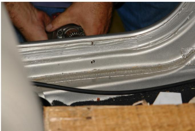
Step 16. Note that the hole exits above the floor in the area on the back side of the sill. The drill guide places the hole at the correct angle to achieve this.
