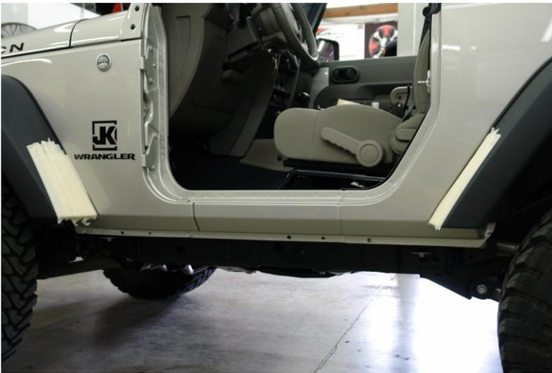
Step 7. Tape off fender flares to protect them from scratches during install.
