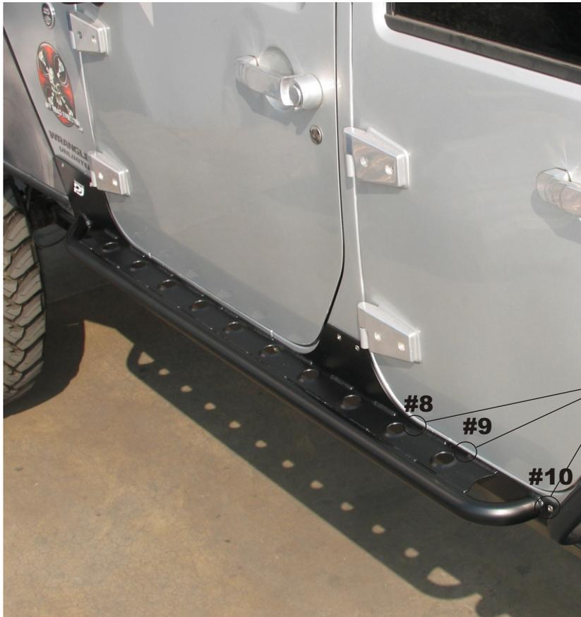
Mounting holes 8,9, & 10 are configured and installed in the same manner using a crush sleeve as as holes 1 through 7.
