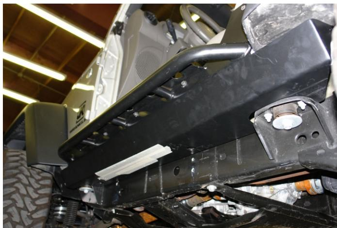
Step 29. After every bolt has been torqued, locate the mounting tabs on each end of the rails. Drill through the hole in the tab with a 1/4" drill bit, and install 1/4 -20 x 3/4" hardware
