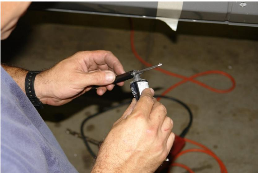
Step 21. Coat the end of the DOM sleeve with a liberal coat of black RTV Silicone before installation.
