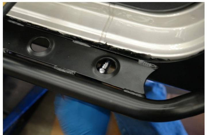
Step 28. After every bolt has been inserted and nuts started on the end of the bolts, begin to torque all of the bolts from the middle mounting points out. Re-torque all bolts in sequence twice.
