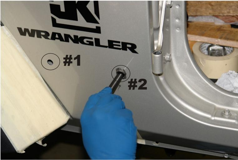
Step 23. Slide the alignment rod into the DOM sleeve and insert all the way through to the hole on the other side of the lower fender area as shown. Hole #1 uses the 3 19/32" length tube. Hole #2 uses the 4" tube.
