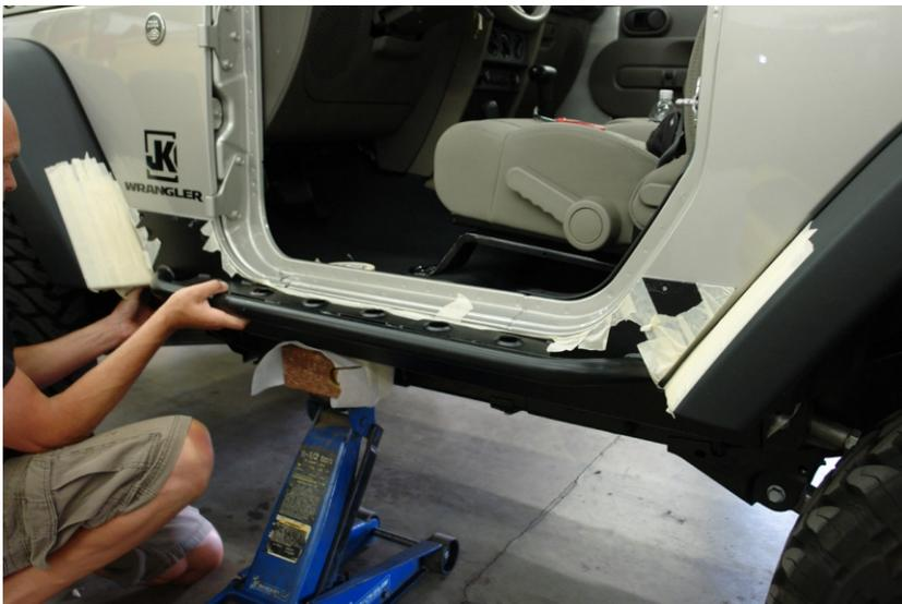
Step 9. Tape the backside of the rail to protect the body of the JEEP, and lift into place.
