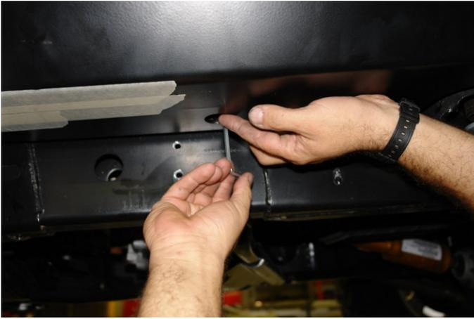
Step 10. Align the holes and bolt the rail into place from the bottom side using the supplied bolts and nut-clips. Use the floor jack out at the end of the tube rail to “cam” or squeeze the rail tightly to body before transferring the hole centers before drilling the body.
