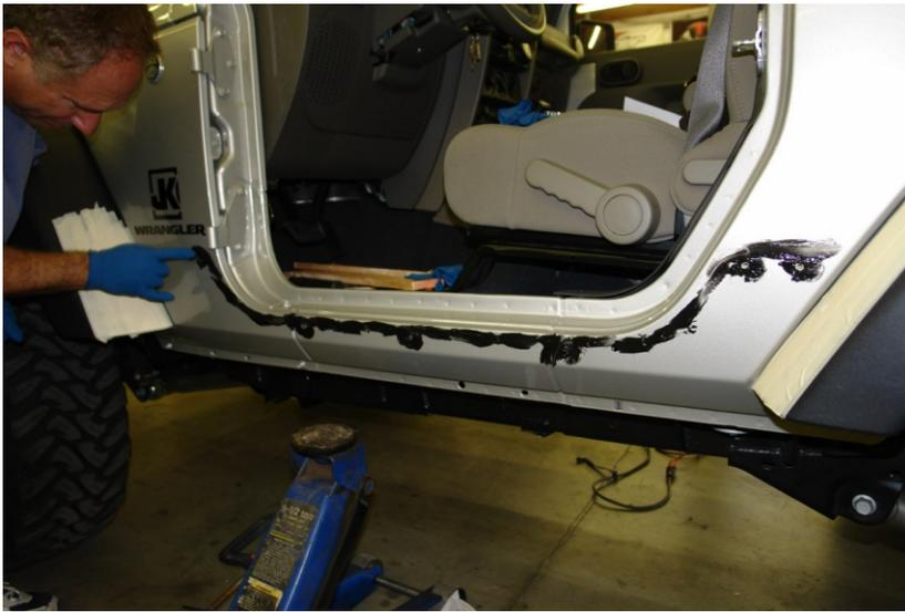
Step 26. Right before final installation of the rails, coat the entire upper contact area of the body with black RTV sealer to prevent leakage of water, sand and grit between the body and rail assembly.
