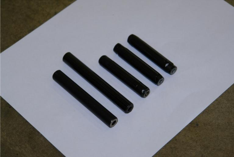
Step 19. Your hardware bag contains 10 DOM sleeves of different lengths. These are to be used as crush sleeves when inserting the 1/4" bolts through the sill plate. At this time, locate and separate all of these by length.
