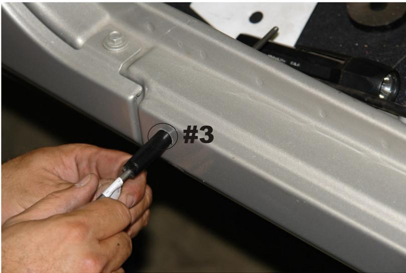
Step 22. Slide the alignment rod into the DOM sleeve and insert all the way through to the hole on the other side of the door sill area as shown. These 3 holes under the door sill area are holes # 3,4,& 5. Use the 2 23/32" tubes in these holes.
