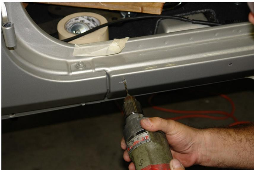
Step 13. After center punching body, begin to drill 1/4" holes at all mounting points. There are multiple layers of sheet metal to drill through to reach the inside wall of the door sill area. Drill **only** the outer layer with the 1/4" drill bit at this time.
