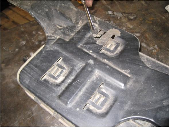
Use a Slotted Screwdriver to pry up the tabs of the factory base plate.
