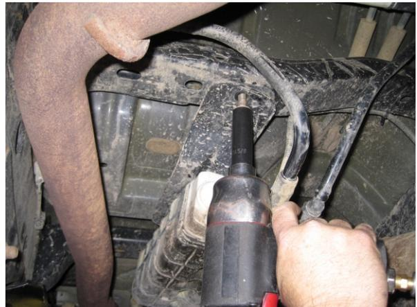
Remove the forward and rear bolts holding the cannister to the crossbrace.
