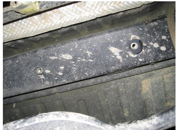
Align Nut-serts with holes in cross-brace. Reinstall the body mount bolt on 4-Door.
