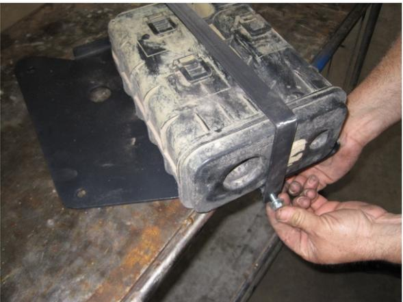
On the opposite end, bolt the two pieces together using the 3/8x 1" bolts, nuts, and flat washers.
