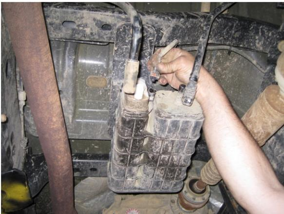
Removing electrical connection wire.
