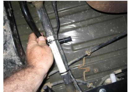
Rotate and route the factory hose over the cross-brace as shown in this series of photos.
