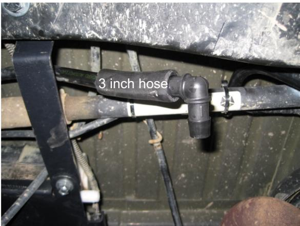
Insert plastic elbow into cut factory tube.
