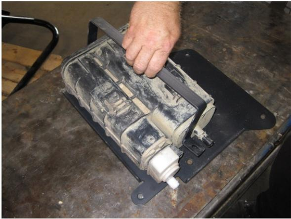
Place cannister on the new PJ skid plate and align bracket with bolt holes.
