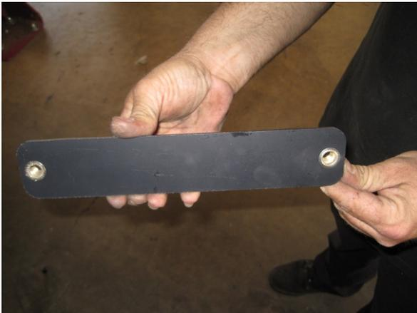
This flat bracket uses two 3/8" dia nut-serts as shown.
