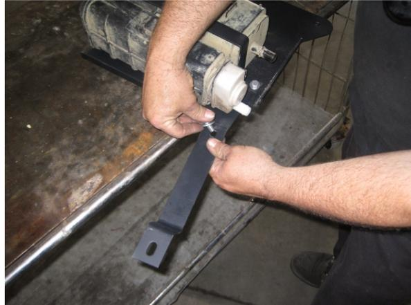
Bolt this bracket to the skid plate as shown using the 3/8x 1" bolts, nuts, and flat washers.
